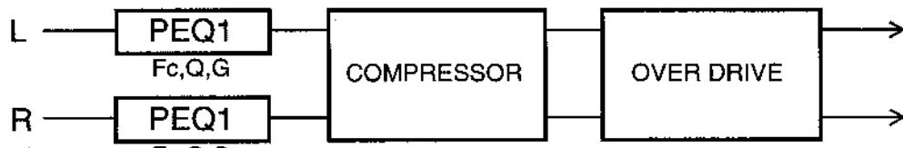
Combines parametric equalizer, compressor, and overdrive.
