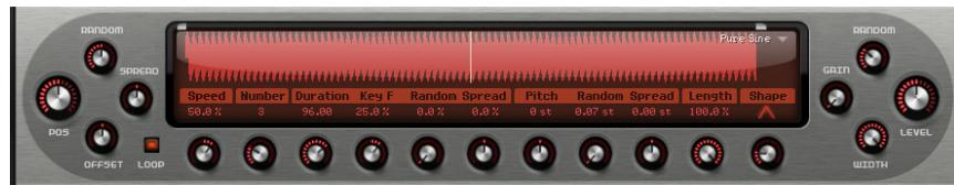
Padshop comes with a large variety of samples that can be used as sources for the grain oscillator. Loading a new sample in the Oscillator section does not change any of the parameter settings for the plug-in.
