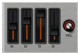
The Velocity control determines how much the envelope intensity depends on velocity. When the control is set to 0, the envelope is fully applied. Higher values reduce the intensity for lower velocities.
