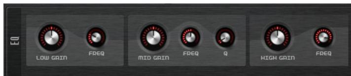
A high-quality 3-band equalizer is available for each layer. The mid-range band acts as peak filter and the low and high bands act as shelving filters. The mid-range band is fully parametric with adjustable gain, frequency, and Q factor.
