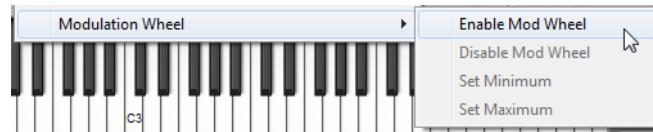
2. On the “Modulation Wheel” submenu, select “Enable Mod Wheel”.
