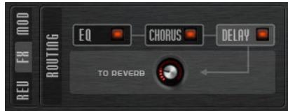
The Routing section shows the signal flow. The signal passes the EQ first, then the modulation effect, and then the delay effect. With the “To Reverb” control, you can specify how much of the processed signal is sent to the global reverb effect.
