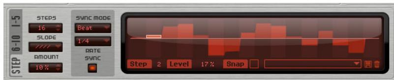
Padshop features a polyphonic step modulator that allows you to create rhythmic control sequences. A sequence can have up to 32 steps.
