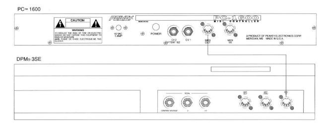
The following diagram illustrates how the PC 1600 connects to a keyboard and rack module, such as the Peavey DPM® 3SE and Peavey DPM® V3:
