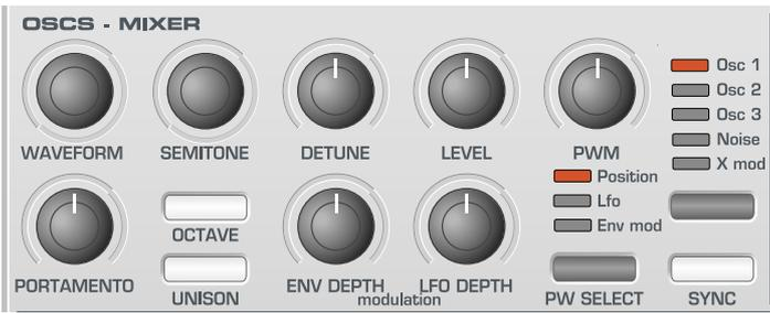
The Oscillator is really the heartbeat of the Synthesizer. It generates an electronic wave (which creates the vibrations). This *Waveform* is produced at a controllable musical pitch, initially determined by the note played on the keyboard or contained in a received MIDI note message. The initial distinctive tone or timbre of the waveform is actually determined by the wave's shape.
