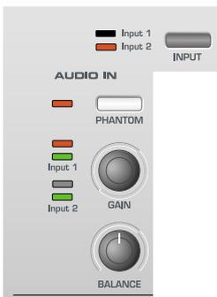
This will set the gain of the preamplifier to the correct level for the Microphone such that it will not distort or be too quiet when recording.
