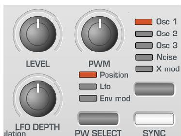
Some synths such as the Novation KS 5 often have a separate Mixer section available on the front panel. On the X-Station's KS Synth implementation, a single LEVEL knob within the OSC / MIXER section is used to adjust the levels of the Oscillators and Noise generator. These may be independently adjusted and mixed together to form a new, more harmonically complex waveform.
