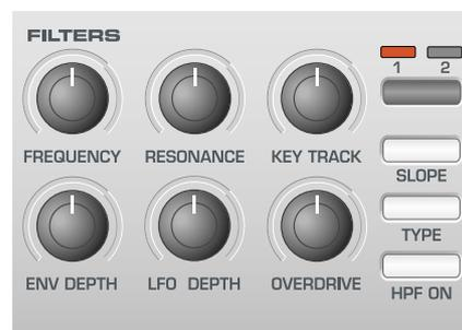
The Filter can be used as a Low Pass, High Pass or Band Pass type.
