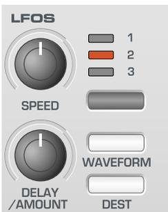
As with an Envelope, the waveforms generated by the LFOs may be fed to other parts of the synthesizer to create the desired movements in the sound.
