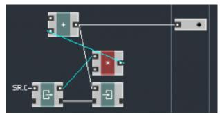
So, first we write, then we read (note that the Read module is clocked by SR.C to make sure that the reading is happening once per audio tick). That makes the read value always one audio sample behind the written one. Now there is no feedback in the structure. Don't see it? OK, let's move the modules around a little bit (we won't change a single connection):
