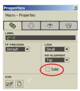
The Solid property tells the Reaktor Core engine whether the macro is to be considered as a solid built-in module for the purposes of feedback resolution or whether it is to be considered transparent. In 99% of the cases, you would want to keep this property on. That's because you typically don't want implicit feedback resolution to happen inside your macros.
