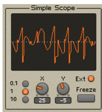
Fig. 6.9 An example of a hard synchronized sawtooth waveform.
