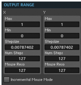
Fig. 1.45 The range and resolution of the XY Module's output values are set in the Output Range area of its Function page.
