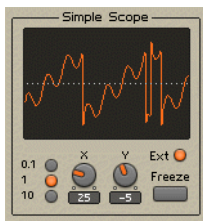
Fig. 6.6 An example of a frequency modulated sawtooth waveform.
