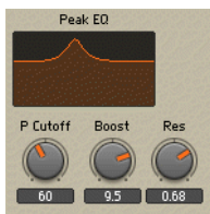
Fig. 10.30 The Peak EQ FM Module's Panel representation with a positive "Boost" value exhibits a positive peak.
