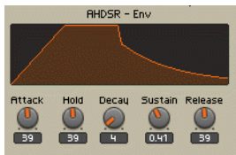
Fig. 9.48 The AHDSR Envelope's Panel representation and knobs for its curve parameters.
