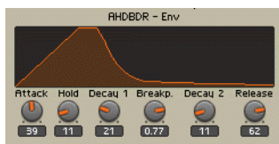
Fig. 9.51 The AHDBDR Envelope's Panel representation and knobs for its curve parameters.
