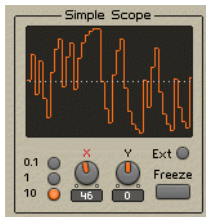
Fig. 6.117 The Random Module is used to generate a pseudorandom signal.
