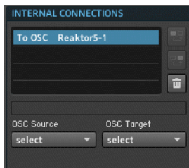
Fig. 15.16 Established OSC Connections appear in the Internal Connections area of the Connections page.
