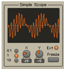
Fig. 6.52 An example of a waveform composed of 4 additive sine waves.
