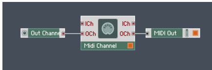
Fig. 14.61 Setting the outgoing MIDI Channel directly from the Instrument Panel.
