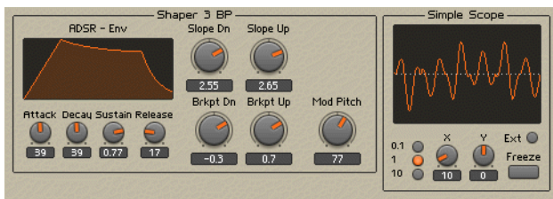
Fig. 12.26 The resulting waveform of a parabolic oscillator sent through a waveshaper with three breakpoints where two slopes are modulated by a sine oscillator with pitch set by the "Mod Pitch" knob.
