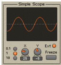
Fig. 6.31 The waveform of the parabol oscillator.
