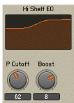
Fig. 10.34 The High Shelf EQ FM Module's Panel representation with a positive "Boost" value.
