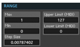
Fig. 2.48 The "Min", "Max", "Lower Limit", and "Upper Limit" values can be set in the corresponding edit fields of the Sel Poly Aftertouch Module's Function page.
