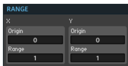
Fig. 1.61 Use the Range area of the Poly Display Module's Function page to set the range of coordinates that are displayed on the Module's Panel representation.
