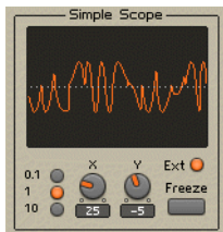
Fig. 6.37 An example of the waveform of a hard synchronized parabol oscillator.
