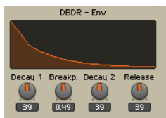
Fig. 9.24 The DBDR Envelope's Panel representation and knobs for its curve parameters.
