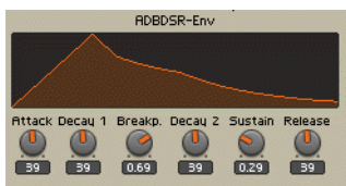
Fig. 9.45 The ADBDSR Envelope's Panel representation and knobs for its curve parameters.
