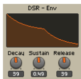
Fig. 9.21 The DSR Envelope's Panel representation and knobs for its curve parameters.
