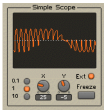
Fig. 6.49 An example of a hard synchronized sine waveform.
