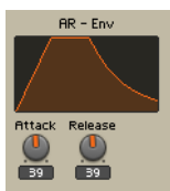
Fig. 9.33 The AR Envelope's Panel representation and knobs for its curve parameters.
