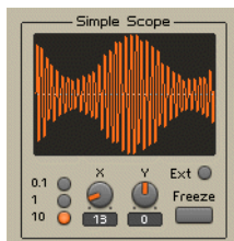
Fig. 9.3 The signal of a sine oscillator to which a tremolo effect has been applied.
