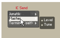
Fig. 15.11 The incoming signal at this IC Send Module has been routed to two faders in the Master Instrument one of which controls the Master Level the other the Master Tune parameters (as indicated by the fader Labels).
