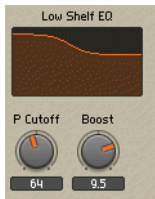
Fig. 10.38 The Low Shelf EQ FM Module's Panel representation with a positive "Boost" value.
