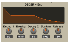
Fig. 9.27 The DBDSR Envelope's Panel representation and knobs for its curve parameters.
