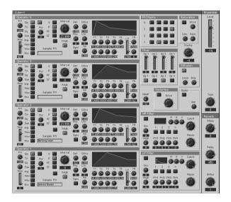
Cube-X is a complex hybrid based loosely on the FM model. Owing to its variety of oscillator types (including sample playback) it can achieve a range of sounds beyond those possible with classical FM synths using only sine wave oscillators. As one example, listen to the "Loop Trick" Snapshots (27 through 32) that use FM techniques to manipulate a beat loop.
