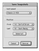
Disk management of Snapshots is handled via Reaktor's File menu. There are separate dialogs for loading and saving Snapshots. Any contiguous group of Snapshot can be saved. Loaded banks of Snapshots can be inserted at any point in the Snapshot list, appended at the end or overwrite existing Snapshots starting with any desired Snapshot. All these actions are subject to the 128 Snapshot limit per bank, however.
