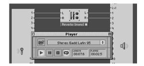
Control Panel and Ensemble Structure for monaural reverb unit. Two types of reverb are featured. The unit is placed between Reaktor's audio input and output Modules to process the playback of Reaktor's Audio File Player (bottom).
