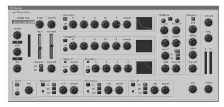
Triptonizer uses another of Reaktor's resynthesis Modules—the Sample Pitch Former. It analyzes the formants (i. e. resonant bands) of small fragments of the sample, then resynthesizing the sound at any pitch, based on that analysis. In other words, it constructs a new waveform based on its analysis of the sample fragment and oscillates that waveform.
