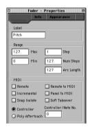
If Incremental is turned on, the incoming MIDI messages will be interpreted as indicating the hardware controller's direction and speed. (This only works with continuously rotating knobs such as those on Native Instrument's 4Control. In that case, incoming values of 64 and greater indicate clockwise motion with higher values indicating higher speeds. Similarly values of 63 and below indicate counterclockwise motion.)
