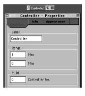
The Properties of the MIDI Controller In Module are shown on the left with those of the MIDI Controller Out Module on the right. For incoming MIDI Controller messages, you set the Controller number, incoming value range (in case the external control does not use the full MIDI range) and the output range for the Module. Like a Control Panel control, the MIDI Controller In Module also has a Soft Takeover mode and
