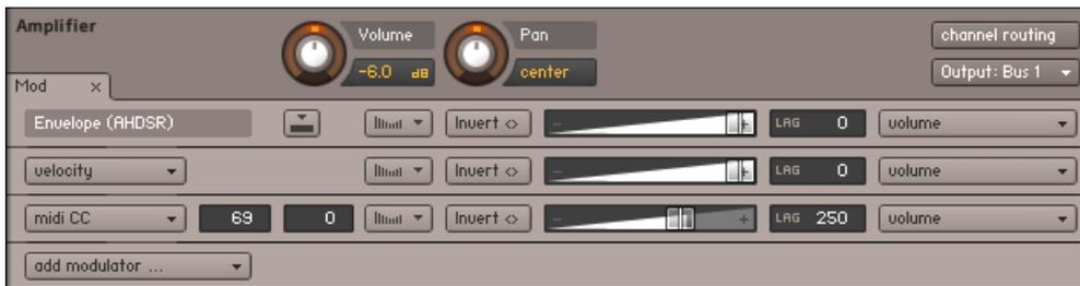
The Modulation Router of an Amplifier Module.
