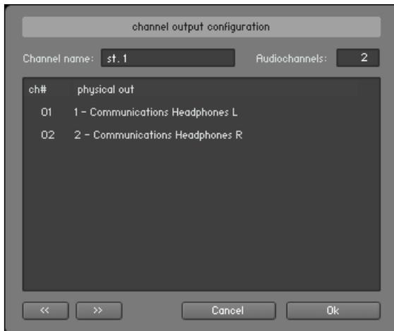
In the Channel Configuration dialog, you can adjust the number of audio channels and the respective physical output assignments.
