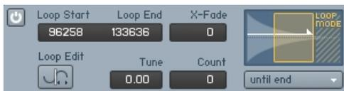
The detail view allows you to adjust the start and end positions of your loop regions numerically with sample value accuracy.
