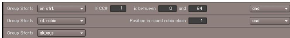
Multiple Group start conditions, combined with “and” operators. This means that all specified conditions must be met before the Group becomes active.
