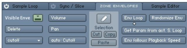
From left to right, the Zone Envelopes tab provides selection and delete functions, assignment buttons, edit tools, and utility functions.
