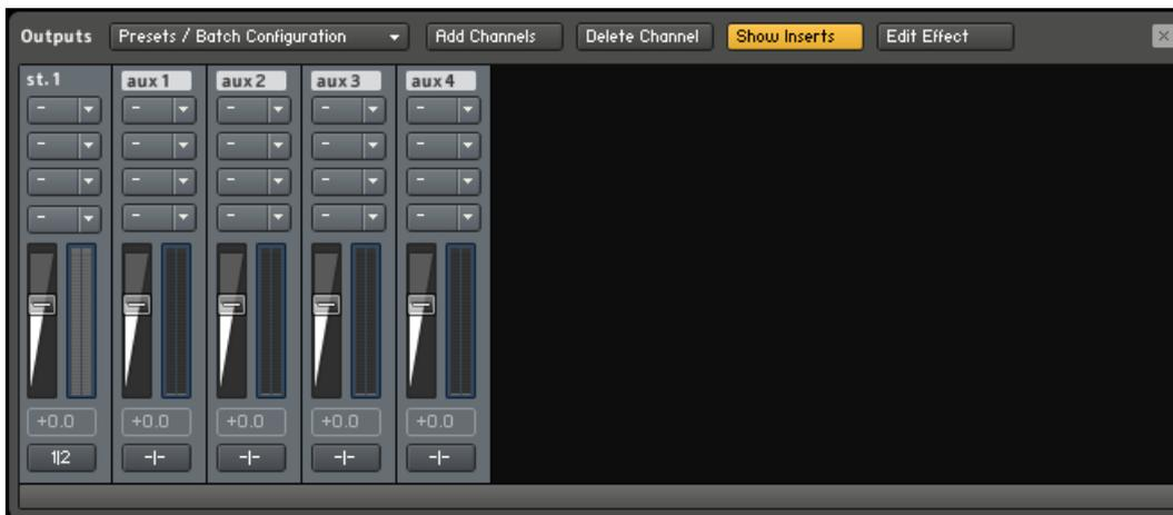
The Outputs section, displaying a stereo Output Channel strip at the left, and the four Aux Channel strips at the right.
