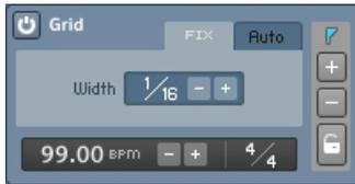
The Auto mode detects peaks in your Sample and uses these for slicing.
