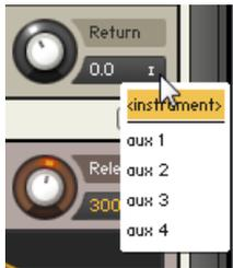
Changing the output assignment of your send effects modules allows you to isolate wet effect signals from your Instrument's Output Channel.
