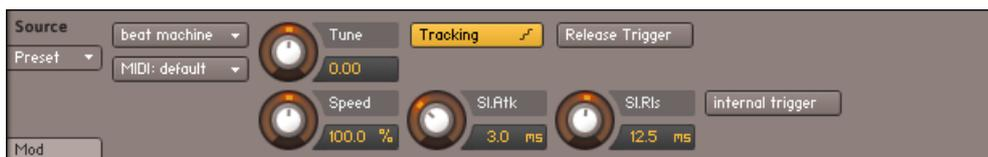
The Beat Machine mode shouldn't be activated manually; it's better to Slice your Samples first in the Wave Editor and then activate it via the Use Beat Machine button on the Sync / Slice tab.
