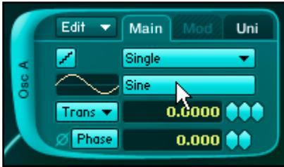
The Waveform Selector of our first Oscillator, currently displaying *Sine* (the loaded Waveform).
