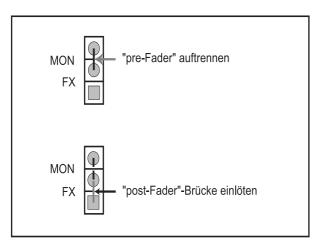
Abb. 5.1: Modifikation MON/FX "pre-Fader" > "post-Fader"
