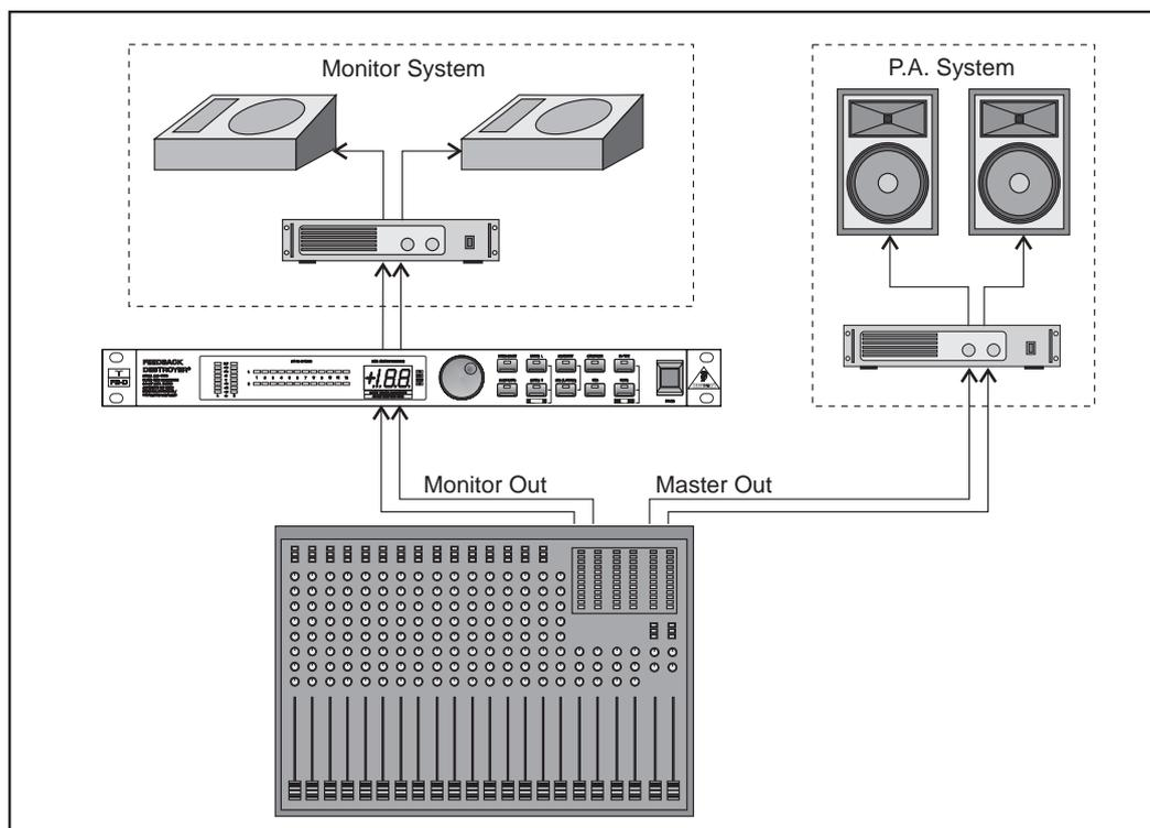
Fig. 3.1: Using the FEEDBACK DESTROYER PRO in the monitor path
