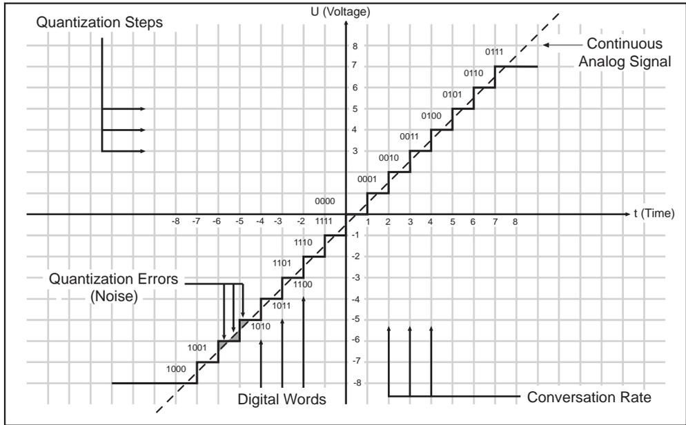
Fig. 4.4: Transfer diagram for an ideal linear ADC (2's complement representation)
