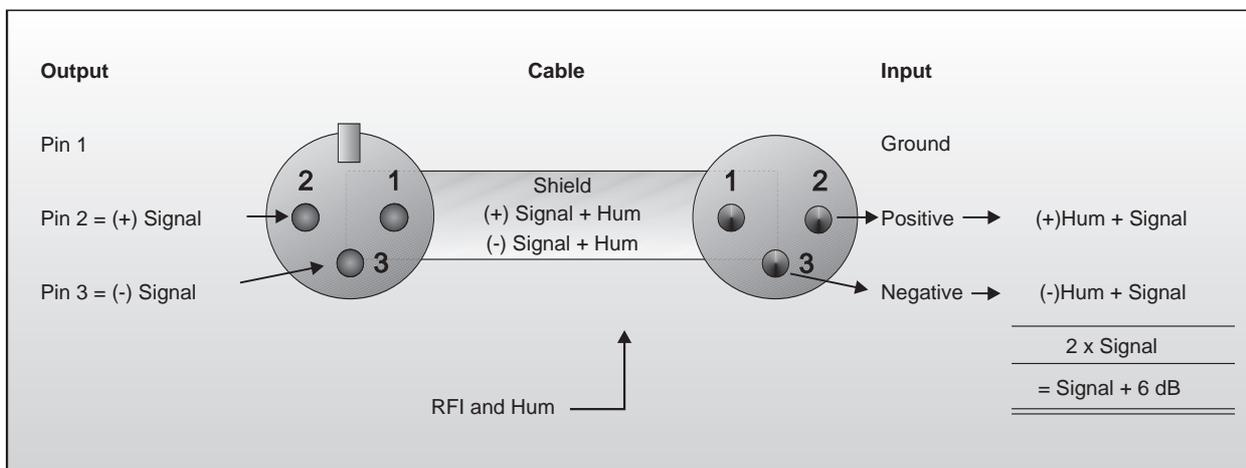
Fig. 5.1: Compensation of interference with balanced connections
