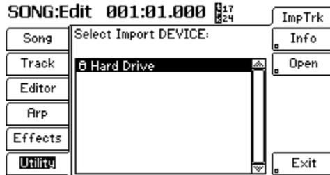
You should see the Fusion Hard Drive. Make sure it is highlighted and press **OPEN**.
