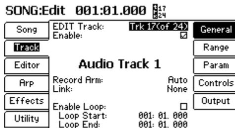
Since our *Record Arm* parameter is set to Auto, we must actually select the audio track we are recording to on the Track page to arm it. If this parameter was set to ON, the track would not have to be selected. It would be record ready from any menu.
