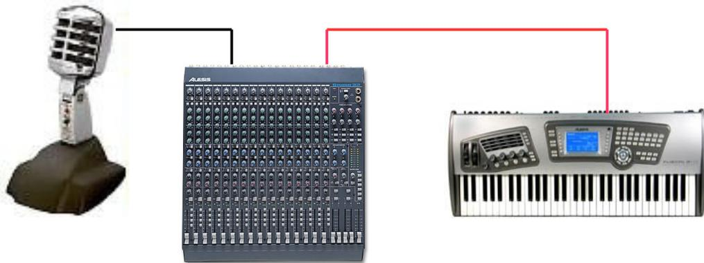
Believe it or not, you can even use the Fusion as a stand alone digital 8 track recorder. Using a mixing console with 8 direct outs/busses or a dedicated 8 channel mic pre, you can record your entire band live. Those tracks can then be exported as .wav files to your computer for further editing or mixing!
