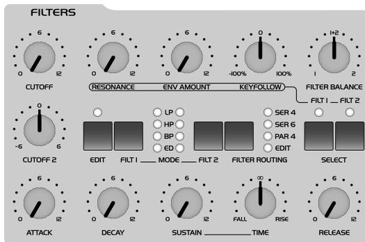
Locate the *CUTOFF* pot (not to be confused with *CUTOFF 2*!) in the section labeled *FILTERS*, directly above the section labeled *AMPLIFIER*. Rotate the pot to the left and right and note how the sound
