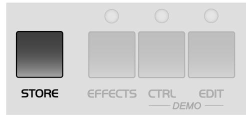
■ *To belabor the point, when you store a MULTI program, only the content of the MULTI edit buffer is saved, not however the sound programs in the PARTs. These must be stored individually in MULTI SINGLE mode.*
