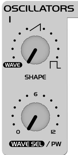
In the sound program, SHAPE is preset to the center position (12 o'clock), which is equivalent to a value of 64. On the pot, this position is identified via a graphic depiction of a sawtooth wave. You can definitely see why this waveshape bears the name "sawtooth." Press and hold a key and slowly turn the pot clockwise. You should be able to hear how the tone becomes increasingly more hol-
