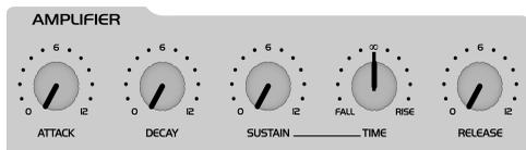
Rotate the *ATTACK* pot while you repeatedly engage a key to hear the note. The further you turn the pot up, the longer it takes for the sound to achieve maximum volume after the start of the note. So you can say *ATTACK* controls the initial volume swell of the sound.
