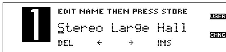
2. At this point, if you wish to change the program name, you can use the parameter <1> button to delete character spaces. The <2> and <3> buttons to select the character position. The <4> button is used to insert character spaces and the <Program/Data> wheel to change characters.
