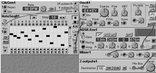
The clock generator delivers a trigger signal. It switches the sequencer to the next step and simultaneously triggers the ADSR envelope.
