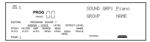
The Assign Voice function is the most fundamental part of Program editing. It is where you choose the particular sample that forms the basis of a sound. To avoid scrolling through long lists of samples (remember, there are 20 megabytes of sounds in here!), sounds are divided into groups. After selecting the group, you then select the sample within the group.
