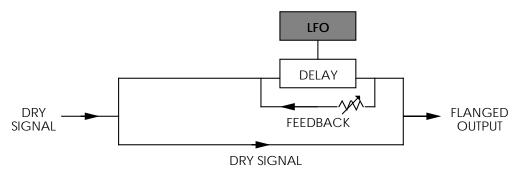
Many variables are available, from varying the speed and depth of the LFO to feeding back part of the signal to make the effect stronger. The Flanger's waveform shape can be either "Normal" or "Inverted". Use the "Inverted" setting for a more dramatic flange effect.
