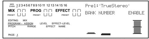
Note: This illustration shows a Mix with all 16 MIDI channels enabled. If a channel is not enabled, its number will not show in the display unless the MIDI cursor is under the number.
