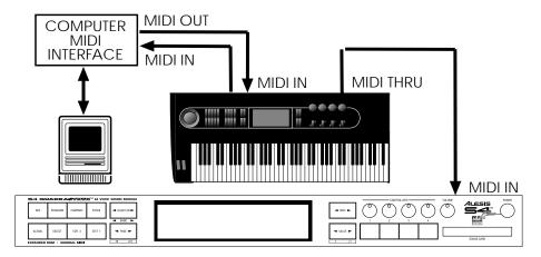
If you are driving other MIDI gear (such as an expander module or MIDI-responsive signal processor), you'll usually drive these from the sequencer if it has additional MIDI outputs. However, you can also use the S4 Plus's MIDI THRU connector to drive other modules since the Thru carries a replica of what appears at the S4 Plus's MIDI IN, which is the same as the sequencer's MIDI OUT.
