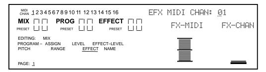
Quad Knob [4] (FX-CHAN) lets you select which Channel (1—16) of the Mix whose Effects Patch you wish to use. If you set the Effect Channel to 1, the Mix will use the Effects Patch used by the Program on Channel 1. The Effect Channel is also used to determine what MIDI channel the Effects Patch will be set to for receiving MIDI controller information for the Modulators (see the Mod section later in this chapter for more on real-time MIDI control).
