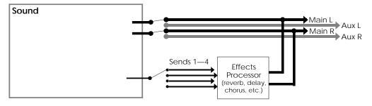
Effects parameters are edited separately from either the Program or the Mix, using Effects Edit Mode (more in Chapter 7). In Program Edit Mode, each of the four sounds in the Program has its own Effect Level control and can be assigned to any
