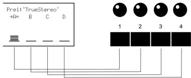
When in Program Edit Mode or Mix Edit , the Quad Knobs are linked to the parameters that appear in the right side of the display. The lower line of the alphanumeric display will show the abbreviated name of each parameter, with a bar graph below it representing the current setting of the parameter. By turning Quad
