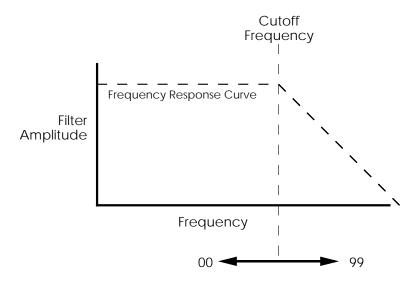
The cutoff parameter changes the frequency at which the highfrequency response starts to roll off. Lower values give a lower cutoff frequency. A value of 00 will cut all sound off.
