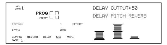
Depending on the selected Configuration, the order of the effects will differ (for example: in Configuration #1, the order reads Pitch, Delay, Reverb; but in Configuration #2, the order is Delay, Pitch, Reverb).
