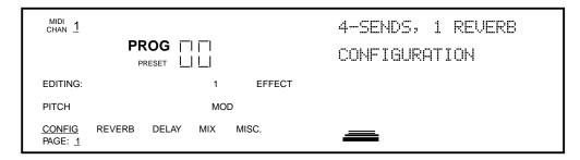
Quad Knob [1] selects the Configuration. As you scroll through the various Configurations, each one's name will appear in the upper right section of the display.
