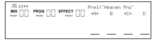
All MIDI channels that are active in the current Mix are shown at the top left, to indicate multitimbral operation. The current MIX and EFFECT numbers are displayed, along with the current Bank and Mix's name. The PROGram number display shows the program assigned to the <u>underlined</u> MIDI channel.
