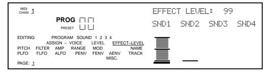
Note: If a Sound is not enabled in a Program, its title will be shown in lowercase ("snd4"), and adjusting its controls will have no effect on the Sound until the Sound is enabled. To enable a Sound, hold down its respective Quadp Button (i.e., [3] for Sound #3) and press VALUE [Æ].
