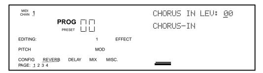
The Configuration has two Reverbs, one on send 1 (which send 2 can share), the other on send 3 (which send 4 can share). There is only one parameter in this page: Chorus Input Level. Quad Knob [1] lets you adjust the level of the signal coming from the Pitch output going into the Reverb, otherwise the signal comes purely from the Pitch input.
